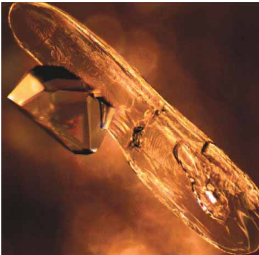
Figure 4: Metastable Form II Piracetam (rough dissolving crystal) undergoing a solution mediated polymorphic transformation to FIII (smooth growing crystal) 6
